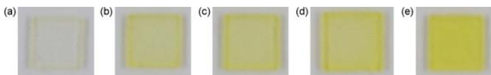
Figure 1.2.14 Photographs of acetylacetone impregnated sensor element before and after exposure of formaldehyde: (a)
