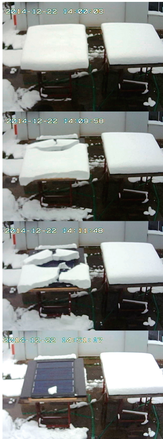
Fig. 8 Field experiment at Daisen, Akita with constant current heating of 12 A (766 W) started at 11:25.
