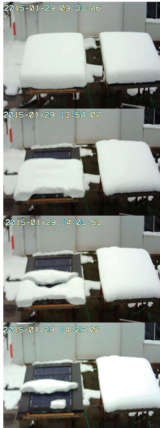
Fig. 9 Field experiment at Daisen, Akita with constant current heating of 6 A (312 W) started at 9:33.
